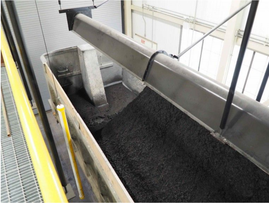
Figure 15: Collected ash from a biomass heating system at General Mills being loaded into a truck bed for transport to local farm fields (Hunt 2017).
