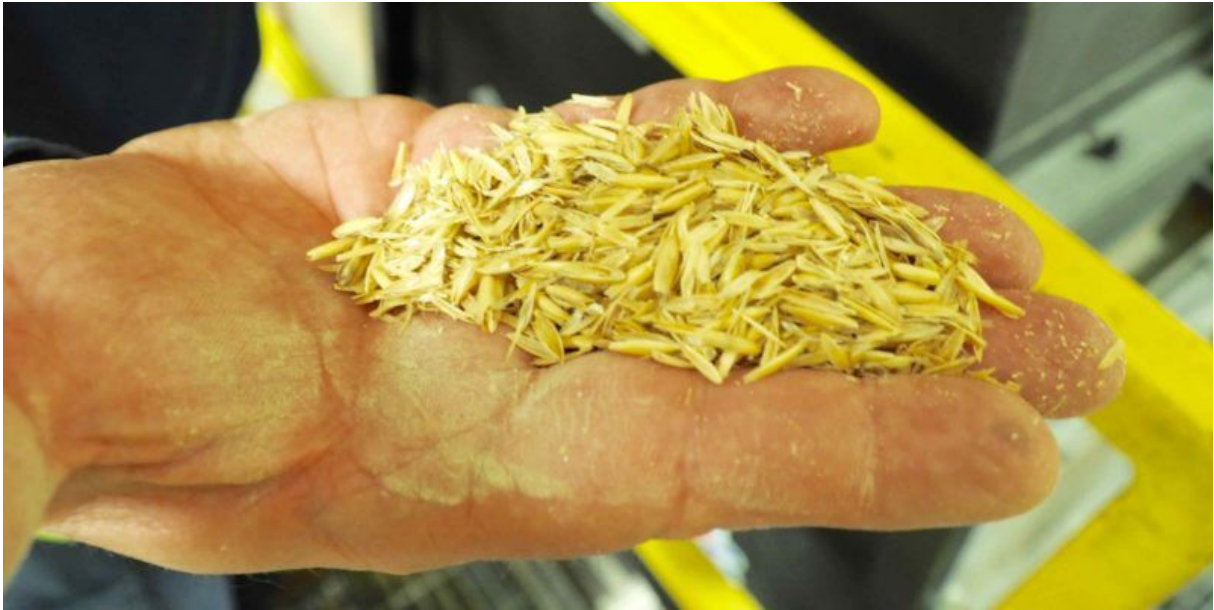
Figure 14: Waste Oat Hulls used in a biomass heating system at General Mills (Hunt 2017).
