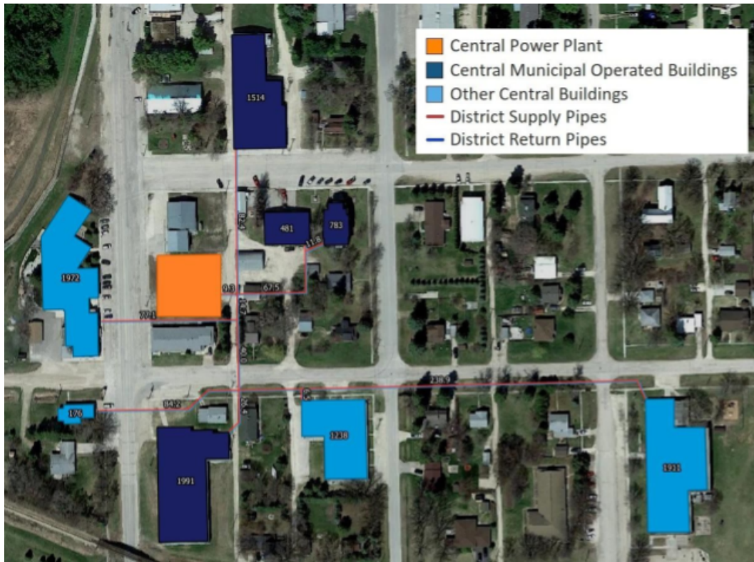
Figure 25: Example network configuration with building polygons in Emerson. Pipe lengths (shown in m) and building polygon area (shown in m 2 ) indicated for the configuration.
