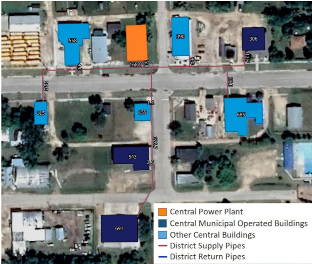
Figure 26: Example network configuration with building polygons in Dominion City. Pipe lengths (shown in m) and building polygon area (shown in m 2 ) indicated for the configuration.
